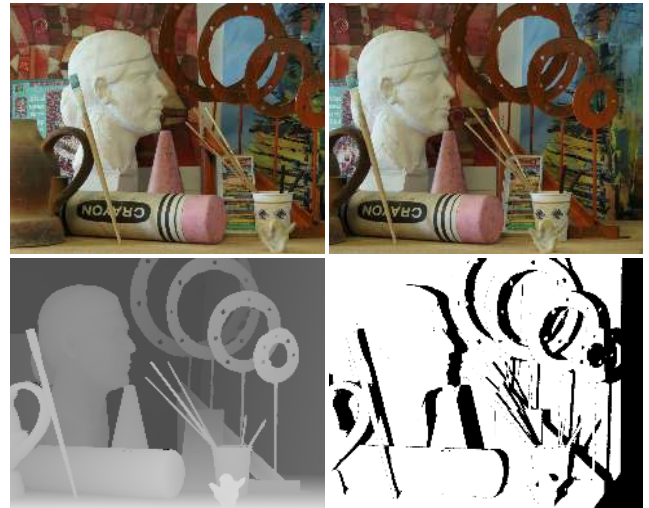
FIGURE 14. “Art” stereo pair. From left to right: left and right views (top), disparity map with holes filling of the right view and occlusion map of the right view. Occluded regions appear in black.
