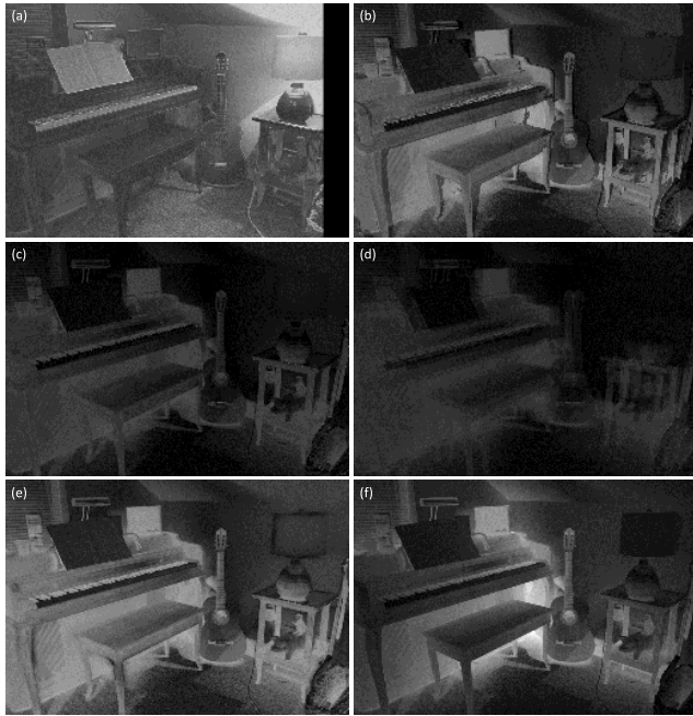
FIGURE 19. JND profiles of “Piano” stereo pair obtained using different 3D-JND models. (a) BJND map, (b) JJND map, (c) MJND map, (d) SJND map, (e) HJND map, (f) DJND map.
