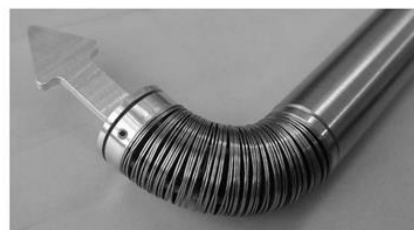
Fig. 13. Steerable tip and ring-spring version I with diameter of 15 mm [21]
