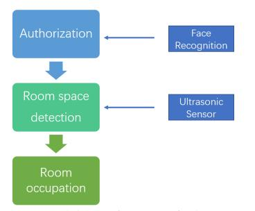
Figure 4. The block diagram for the process of study room occupancy [89].
