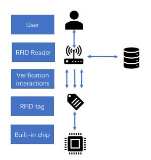
Figure 9. The workflow of smart RFID authentication system structure [108].
