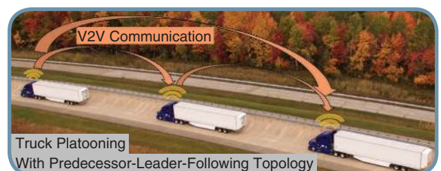
FIG 3 CACC for heavy-duty trucks: “Truck platooning”.
