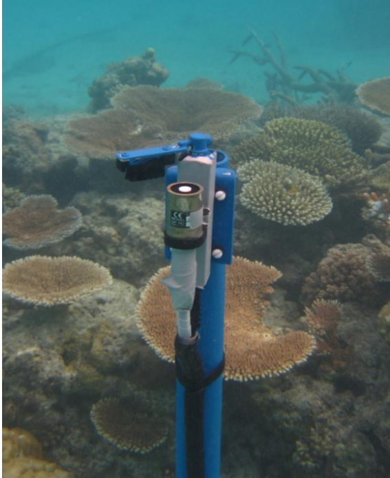
Fig. 4. Light meter with wiper on top to clean accumulating algae periodically [9].
