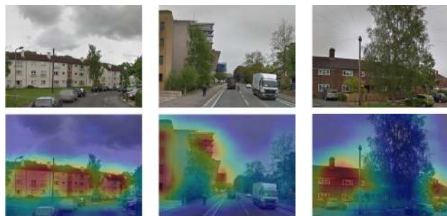
FIGURE 6. Examples of images from urban environment (top) and the attention scores (bottom) generated by the AdAGeo architecture [168] which implements attention via class specific activation maps. The attention is focused on building, disregarding dynamic objects, uninformative areas (sky) and objects that are not stable over time (trees).
