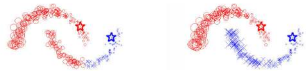
FIGURE 4. Example of diffusion. Left) retrieval from two queries using a nearest neighbour search. Right) the diffusion process allows better capturing the underlying data manifold. Image from [139], Copyright ©2013, IEEE.
