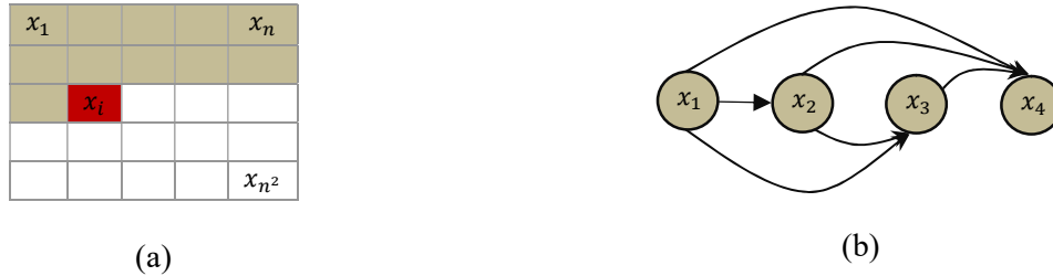
Figure 3: Autoregressive models train a network that models conditional distribution of each pixel given all previous pixels. The image is processed pixel-by-pixel in (a) Raster scan order and (b) Sequentially predicts pixels.
