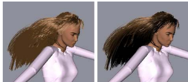
Fig. 26. Interactive hair self-shadowing processed by accumulating transmittance values through a light-oriented voxel grid [80]. (left) Animated hair without self-shadows; (right) Animated hair with self-shadows.
