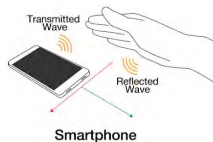
FIGURE 13. Recognize hand gestures by using the ultrasonic signal based on a smartphone [42].
