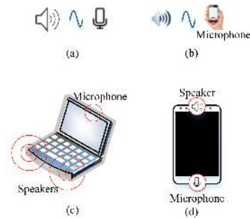
FIGURE 1. Four types of ultrasonic signal-based recognition. (a) Deploying sound sensors in the environment. (b) Utilizing the only microphone built in smartphone. (c) Using a laptop or desktop. (d) Using speakers and microphones built in smartphone.
