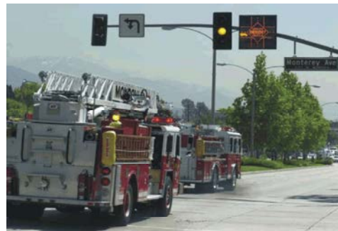
Fig. 6: Monrovia, California fire trucks equipped with emergency vehicle preemption and visual warning system.
