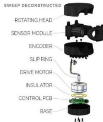
Figure A1. Exploded view of Scanse Sweep 2D LiDAR design [45].
