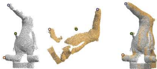
Figure 10: Example of the alignment procedure in 3D for two partial scans of the Coati model (shown to the left): three points are sampled on each scan (the colored dots) and a rigid transformation is derived. If the transformation aligns the largest possible number of points (to the right), then we have found the transformation sought [AMCO08].
