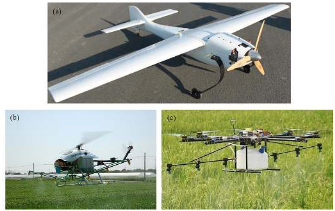
Fig. 9. (a) Fixed-wing UAV, (b) single-rotor hydraulic UAV, and (c) multi-rotor electric UAV. Currently, electric multi-rotor UAVs have a major market share due to their low cost, low failure rate, simple operation, and environmental protection.
