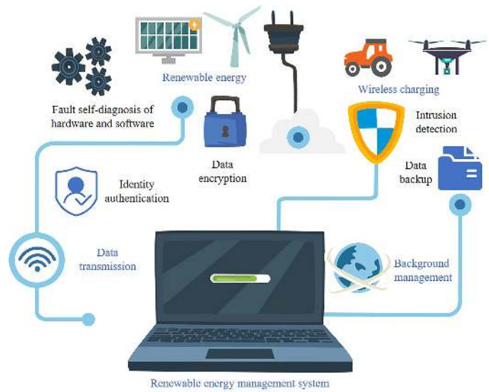
Fig. 19. The security scheme of renewable EMS, including 1) fault self-diagnosis of hardware and software in agricultural facilities and renewable energy equipment, 2) identity authentication and data encryption in data transmission layer, 3) intrusion detection and data backup in background management.
