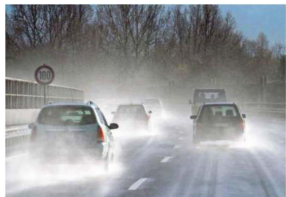
Fig. 8 Water mist splashed by vehicle tires
