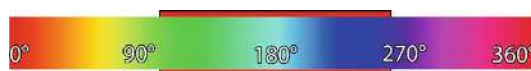
Fig. 2 The hue values (of HSV color space) where a manually selected interval of non-skin colors in swimming videos is highlighted by a red border around the respective colors. The size of the remaining interval reflects the difficulty of defining a skin color interval manually. Image is a reworked version of an image from [29]
