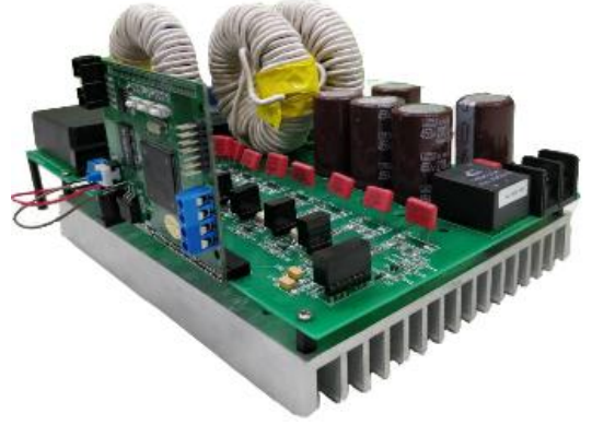
Fig.12 Prototype of the SCIB converter.
