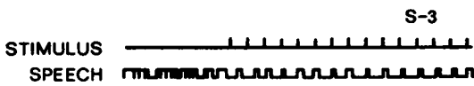
Fig. 6. Sample event recording of a subject reading aloud at the time that the stimulus beat was introduced. The speech pen was activated by the output of a voice-operated relay. The stimulus is vibrotactile and occurs every 0.9 sec.
