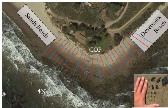
FIGURE 27: Location of transects 1-12 for COP and coverage by 2 m quadrats as used in beach tar surveys. Inset: example images of tar ball size classes 1-5.
