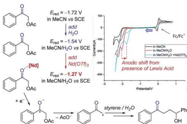
Fig. 4 Effect of the binding of \text{Nd}(\text{OTf})_3 to a ketone on the redox potential facilitating photoredox catalysed reduction, reported by Zeitler and co-workers. Blue arrow in figure demonstrates the direction of the scan, positive current represents oxidation. Adapted with permission from ref. 14. Copyright 2018 The Royal Society of Chemistry.
