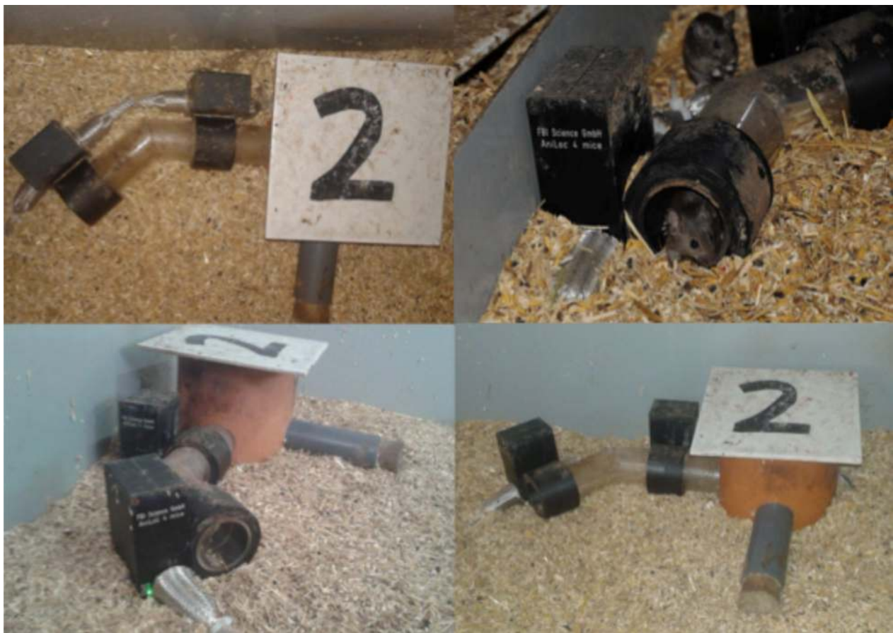
Fig. 3 Mice access nest boxes through acrylic tunnels. Each tunnel is equipped with 2 antennas to allow discrimination between an individual entering or leaving a box. Shown here is (with nest box number 2 as an example) the positioning of the 2 antennas, each connected to an AnilLoc device, with a mouse passing through the “outer” antenna ( upper right ), and a green light signal indicating proper functioning of the device ( lower left )
