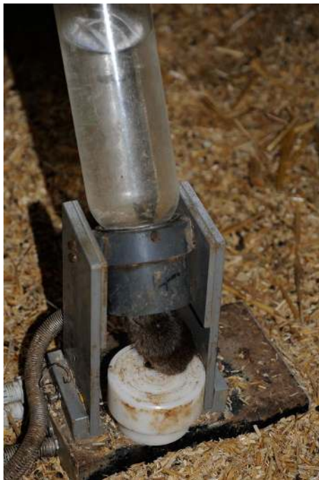
Fig. 4 Intelliscale device (FBI Science GmbH, Germany). A mouse drinks from a water bottle, with its head inside the field of an antenna. It sits on a white , freely movable platform that is connected to a scale in the lower black box. A PIR (infrared motion sensor) is located in the middle of the platform, here partly covered by the mouse
