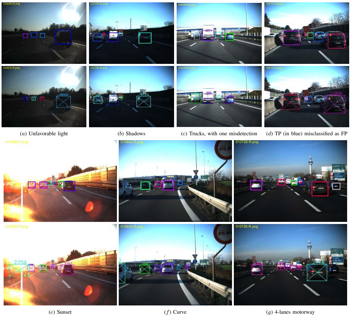
Fig. 6. Representative results on the TME Motorway Dataset. Odd rows show results from our system, even rows the laser scanner generated ground truth. In odd rows, a white bounding box marks a target that has not been validated yet. In even rows, a diagonal cross ( saltire ) marks cars, a vertical ( Greek ) cross marks trucks. A unique color is associated to each ID, as can be appreciated in the complementary video.
