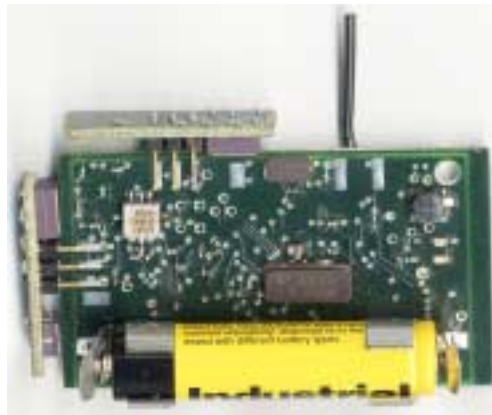
Figure A-5: Back side of main board with daughter boards mounted
