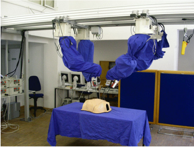
Fig. 1. The EndoPAR system. The four ceiling mounted robots are shown with an artificial chest on the operating table to test tele-operated and autonomous surgical procedures. Three of the robots hold laparoscopic gripper instruments, while the fourth manipulates an endoscopic stereo camera that provides the surgeon with images from inside the operating cavity. The size of the operating area (including gantry) is approximately 2.5m x 5.5m x 1.5m, and the height of the operating table is approximately 1 meter.
