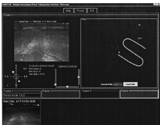
Figure 4. Remote operator interface. Operator interface showing focused view of a single tractor during playback, including video, status, and location on the map. A global map view and focused views for the other tractors are also available.
