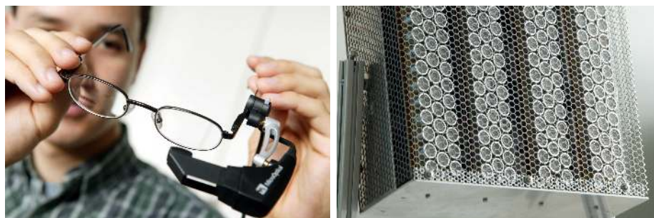
Figure 9.3: Different output devices: Translation Goggles on the left and the Targeted Audio device on the right.
