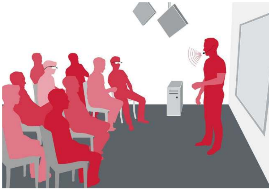
Figure 3.3: The lecture scenario. The speaker in front of the audience is recorded with the help of a microphone. The speech is transferred to the simultaneous translation system running on a PC or laptop and translated. The figure shows also different possibilities of how the translation output can be delivered to the audience: as subtitles on the projection screen, by using loudspeakers, or projected into heads-up display goggles.
