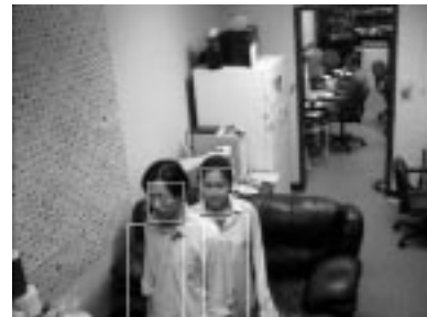
Figure 8. This is a view from one of the static cameras when two people cross paths. Tracking continues despite occlusions.
