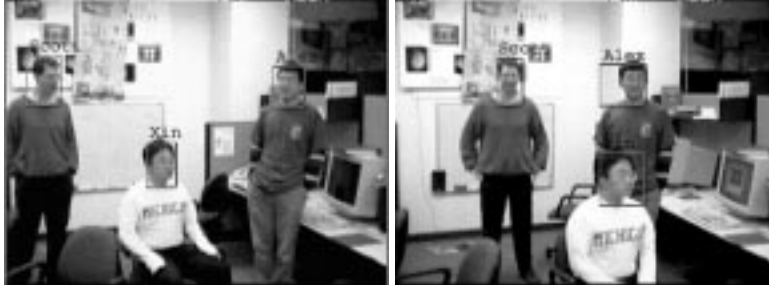
Figure 4. An earlier implementation of our system tracking and identifying 3 people in a scene using only two static cameras. People are recognized by the color of their clothes. Note that in such images face recognition is very hard as each face image has a resolution of about 25x40 on average (the image size is 320x240).
