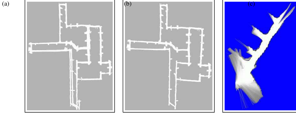
Fig. 3. (a) Map of the coal mine in Bruceton, PA, based on scan matching. This map is obtained by incremental scan matching, and the resulting poses form the input to our loop closing algorithm. (b) Map obtained using our loop closing routines. This map measures approximately 250 by 200 meters in size and contains three large loops. (c) 2-D map of a mine in Burgettstown, PA.
