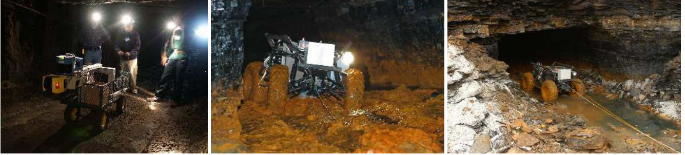
Fig. 1. From left to right: Mine mapping cart with four laser range finders, pushed manually through a mine. Groundhog robot used for breaching difficult mine environments. Strip mine in Burgettstown, PA. None of the vehicles provide any odometry information.
