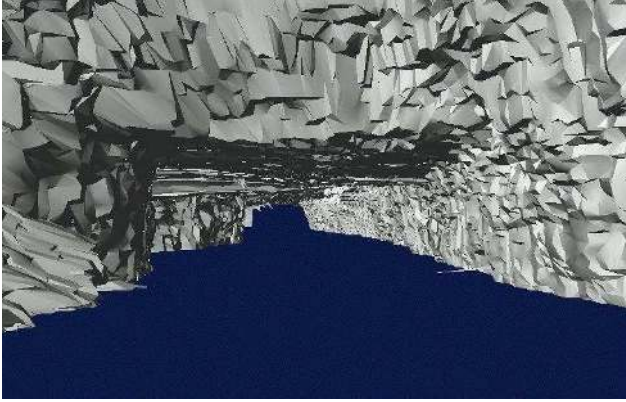
Fig. 7. A section of the 3-D map produced by the Groundhog robot in the Burgettstown mine. This robot possesses no downward pointed laser; hence the map only shows the ceiling and upper side walls of the mine.
