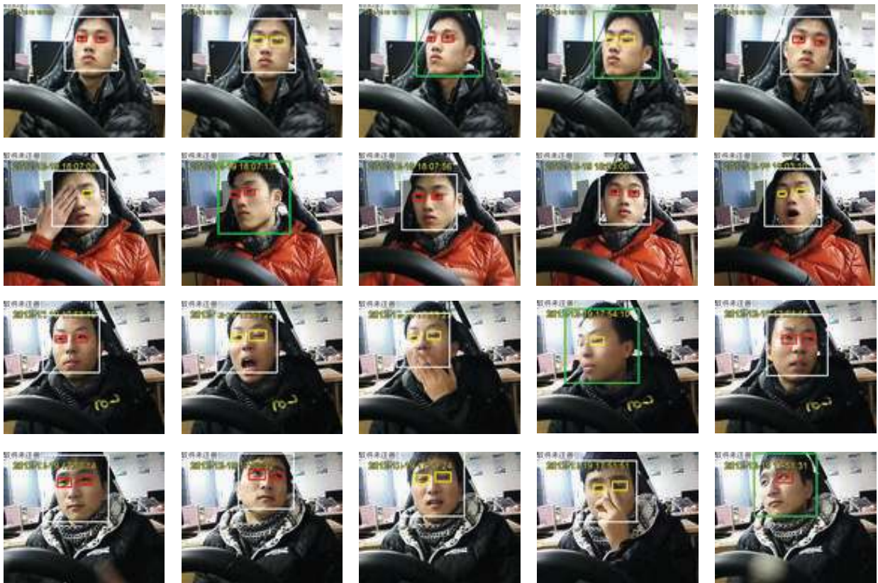
FIGURE 7: Results of eyes location and state recognition.
