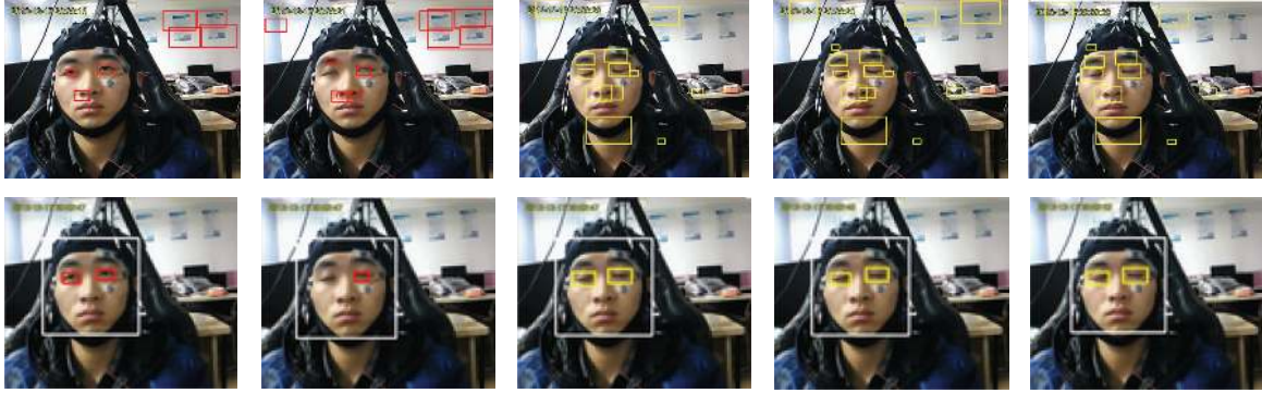
FIGURE 8: Comparison results with our method and the traditional method. The frames of top row are detected by direct Adaboost training eye classifier, while the frames of bottom row are detected by our improved method.
