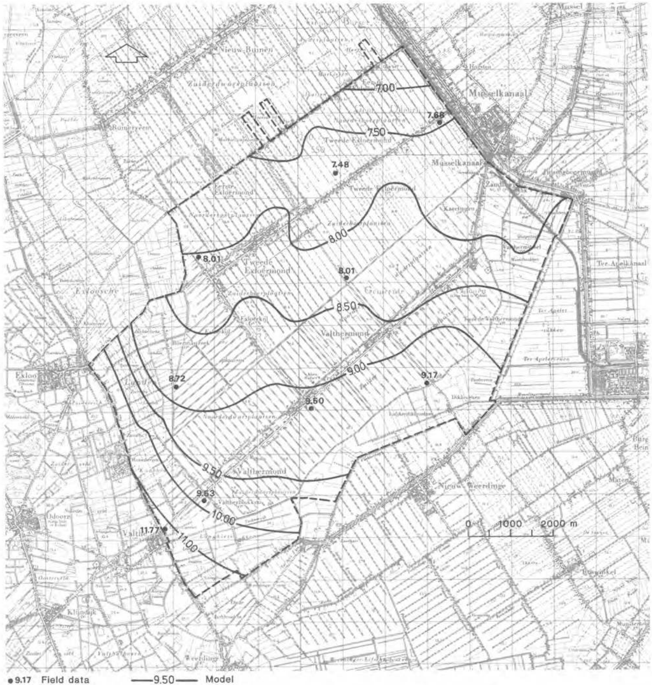
Fig. 6.5. Contour lines of h_2 -values simulated with calibrated parameters and field observations
