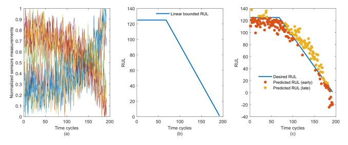
**Figure 4.** Illustration of data behavior in a single life cycle (i.e., cycle1 from FD001) from C-MAPSS dataset: (a) Run-to-failure sensors measurement during gradual degradation; (b) Defined RUL targets for life cycle; (c) Early and late RUL predictions resulted from the target curve fitting with a linear model.
