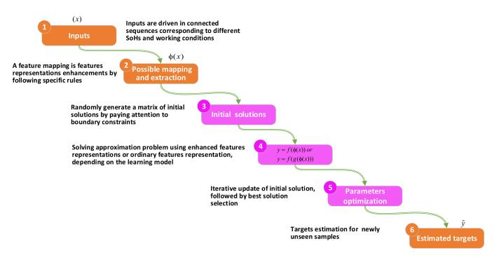
Figure 13. Overview of using ECT and SI within ML models.
