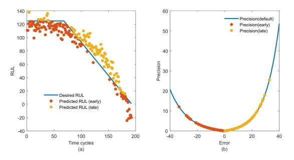
**Figure 8.** Applying PHM 2008 accuracy analysis formula on RUL curve fit: (**a**) RUL curve fit with ML linear model; (**b**) Predictions distributions according to PHM 2008 accuracy formula.
