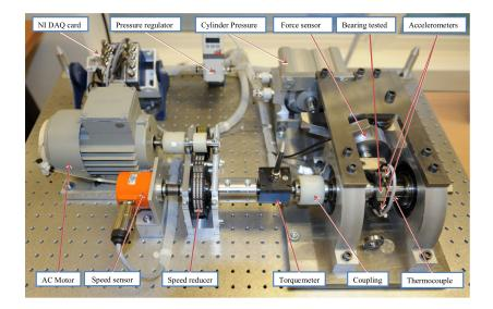
Figure 5. Illustration of the PRONOSTIA platform [25].
