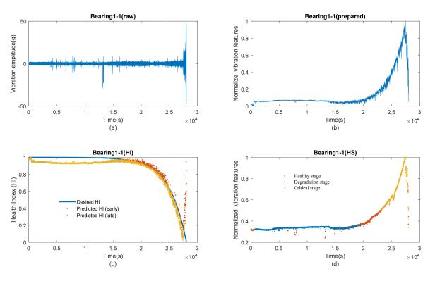
**Figure 6.** Example of health indicators in a single life cycle from PRONOSTIA dataset (i.e., "Bearing1-1"): (**a**) Raw run-to-failure vibration signal; (**b**) Prepared version of the signal; (**c**) Example of HI identification and curve fitting with a linear model; (**d**) HS divisions with GMM model.
