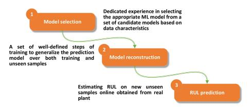
Figure 1. Necessary steps for constructing an RUL prediction model with ML tools.
