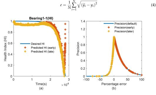
**Figure 9.** Applying PHM 2012 accuracy formula on HI curve fit: (**a**) HI curve fit with ML linear model; (**b**) Predictions distributions according to PHM 2012 accuracy formula.
