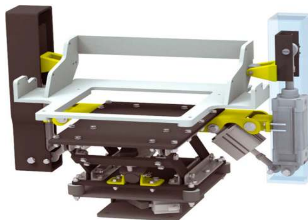
Figure 4. CAD model of the seating suspension structure [43].
