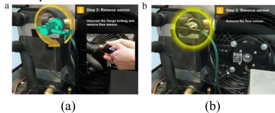
Figure 7. Two types of visualization for the same step in a disassembly procedure. In Figure 8a, “strong guidance”, in Figure 8b “soft guidance”, Weibel [28].
