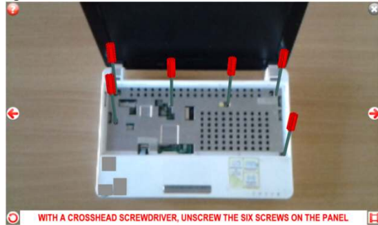
Figure 6. Step by Step assembly procedure by Sanna [23]. Text description of the task is provided on the bottom. Right and left arrows to go forward and backward through the procedure steps.
