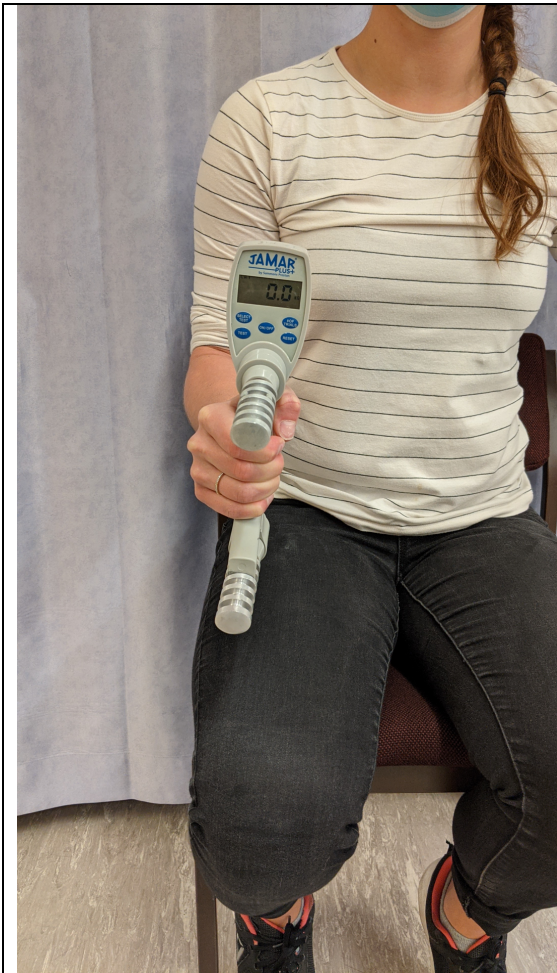
Figure 2B. Dynamometer presented vertically in line with forearm. Hand is positioned with the thumb is around one side of the handle and the four fingers are around the other side.
