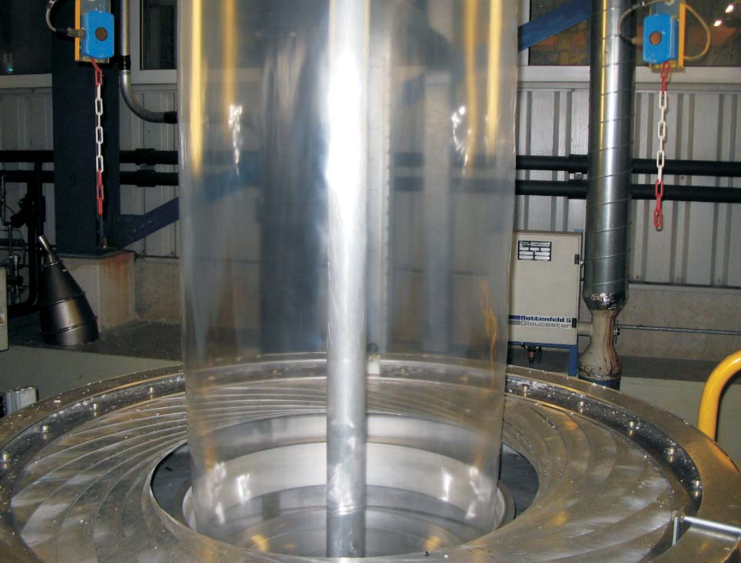
Figure 1. In the industrial film-blowing process shown here, a molten cylinder of polymer is pumped vertically from a circular die, then hauled up in a stream of cooling air as it expands and crystallizes. (Courtesy of Dow Chemical Co.)
