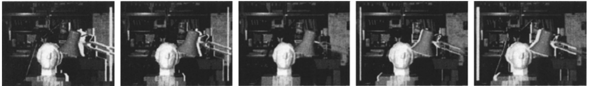
Figure 6. Series of inverse-warped original images. The reference image is the middle one, the matching image is the second from the right. Pixels that are invisible are shown in light grey. Viewing this sequence (available on our web site) as an animation loop is a good way to check for correct rectification, other misalignments, and quantization effects.
