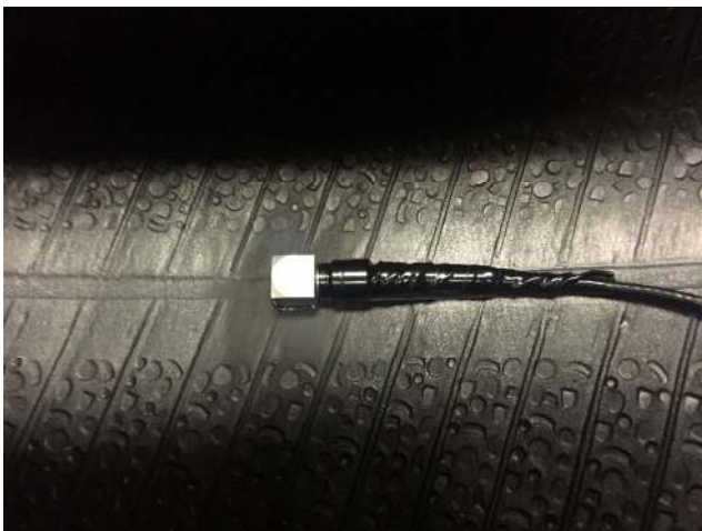
Fig. 5 Using tread sensors (tri-axial accelerometer) to estimate the friction. Reproduce with permission from Ref. [40]. Copyright Khaleghian, 2017.
