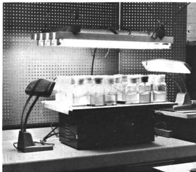
Figure 3. Shaker platform and illumination for incubation
