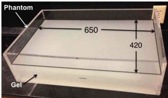
Fig. 11. Rectangular ASTM phantom filled with gel is used in the experiment. The dimensions of the phantom are marked in millimeters.
