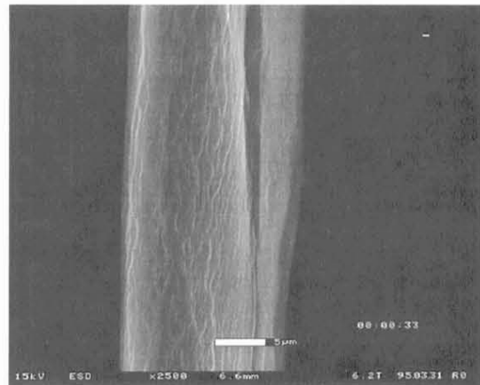
FIG. 4. A digitally captured image of a single wood fiber. The fiber was slowly dried between glass slides to exploit the phenomenon of anisotropic shrinkage. The resulting shrinkage patterns created sufficient image contrast to permit subsequent DIC assessment of surface displacements.
