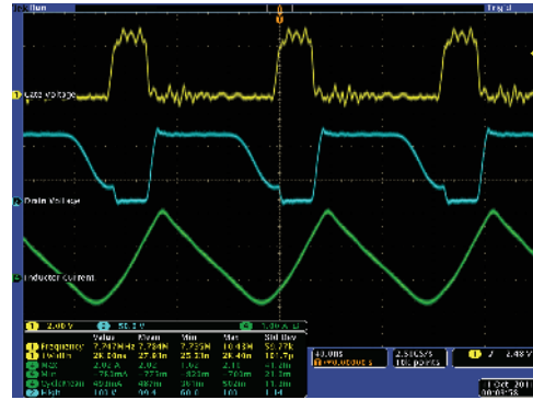
Fig. 5. Waveforms for a prototype HF magnetic stage operating at a frequency of approximately 7.8 MHz from an input voltage of 100 V. Top: Gate voltage (2 V/div); Middle: Drain voltage (50 V/div); Bottom: Inductor current (1 A/div); Horiz: 40 nS/div. At the top end of the input voltage range, the HF stage loses true zero-voltage turn on, but switch turn on is at a sufficiently low voltage that efficiency remains high.
