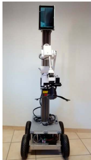
Figure 1. Developed assistive telepresence robot.
