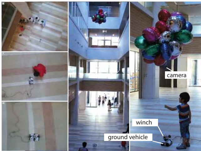
Figure 9: The preliminary implementation of a balloon-mounted camera. Three winches control the distance to the ground vehicle and provide the teleoperator with zoom functionality as shown on the left.
