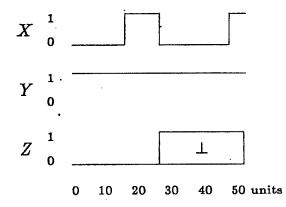
This represents the behavior of the signals X, Y and Z over a period of 50 units of time. The signal X goes up and down twice, while Y is stable with the value 1. Initially Z equals 0 for over 20 units, after which it equals  $\perp$ . Notice that all times are relative. This approach is used because the properties to be examined depend solely on distances between points, independent of any absolute times.
