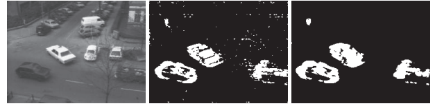
Fig. 2. Tensor-based motion detection on frame 12 of the Hamburg taxi sequence. Motion pixels are marked white. From left to right: (a) original frame, (b) motion detection with |\Omega| = 3^3 , (c) motion detection with |\Omega| = 7^3 . C = 5 was used in all calculations.
