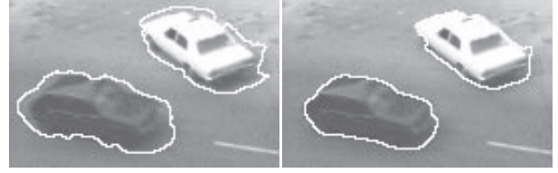
Fig. 4. Contour refinement. Left: motion-based segmentation, right: motion-based segmentation with contour refinement (445 iterations, \tilde{C} = 1.5 ).
