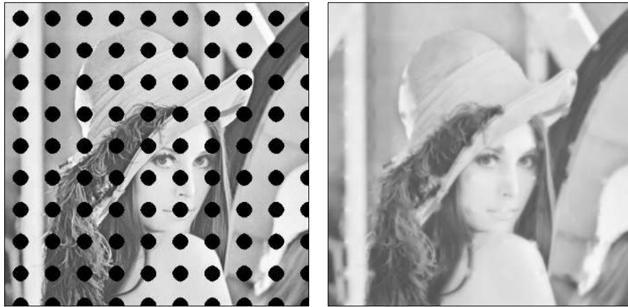
Figure 4.6 Left: Test image. Right: Interpolation using normalized convolution.
