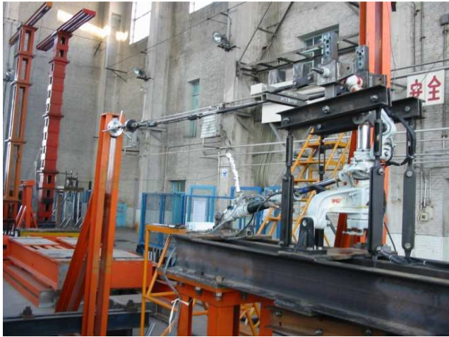
Figure 5. Load calibration of the front landing gear.
