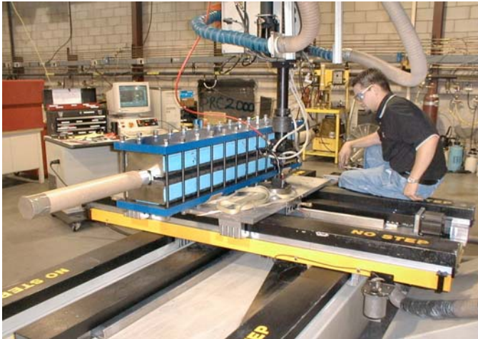
Fig.4. Welding of magnet assembly. Magnet is stationary; laser gun operation allows for automated skip welding through the spacer bar slots and bypassing the press fixture bolts.
