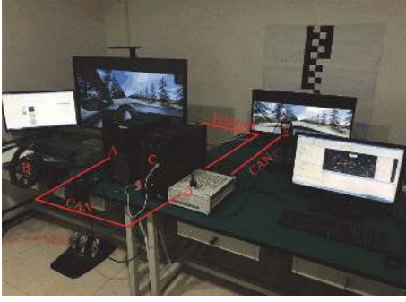
FIGURE 3: Hardware-in-loop test system.
