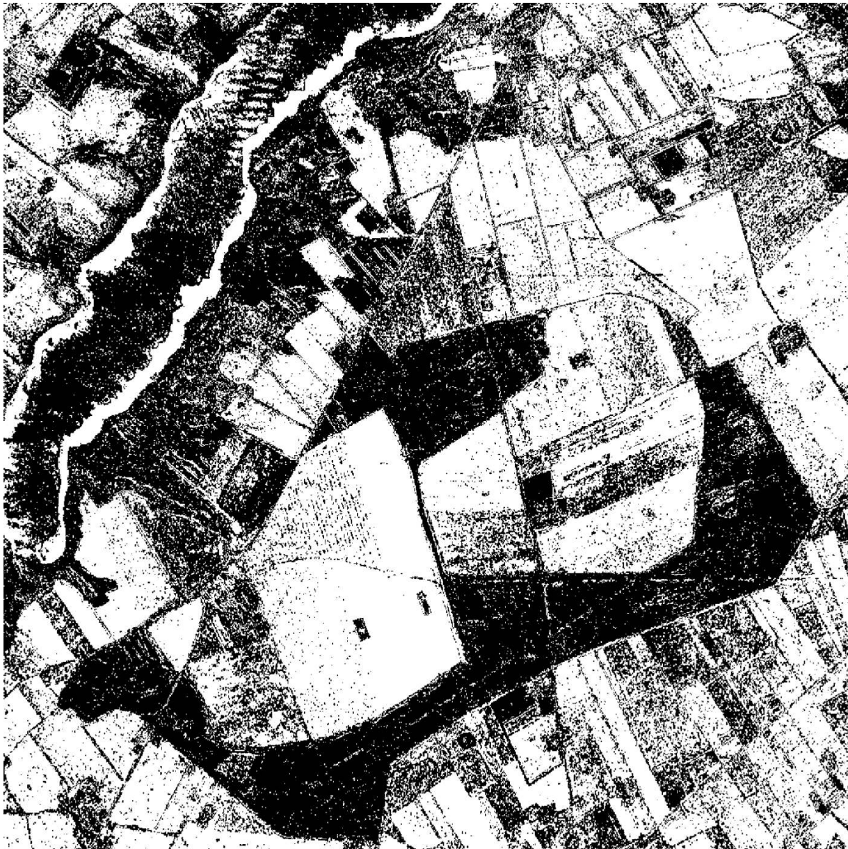
Fig. 10. Rejection of hypothesis of equal covariance matrices at 1% level for the assumed azimuthally symmetric case (white: rejection, black: acceptance).
