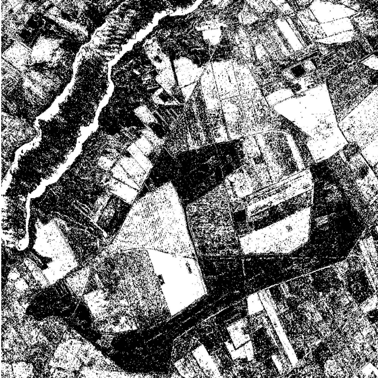
Fig. 11. Rejection of hypothesis of equal covariance matrices at 1% level for the diagonal case (white: rejection, black: acceptance).
