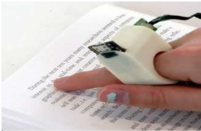
Fig 4: device used to recognize the text and read text for the user.
